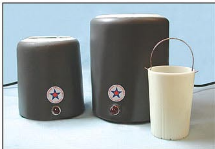
Pickling removes the firescale which occurs during soldering.
